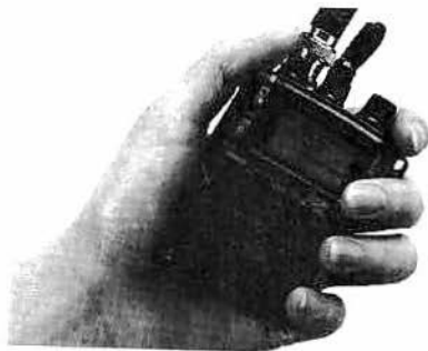
This tiny ICOM handheld transceiver can communicate for 100 miles or more via a repeater. (ICOM Photo)
