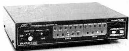
The "PAKRATT-232" from AEA sends and receives most digital modes, even CW.
