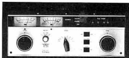
This single-sideband linear power amplifier (the Ten-Tec "Titan") is rated at 1500 watts output.
